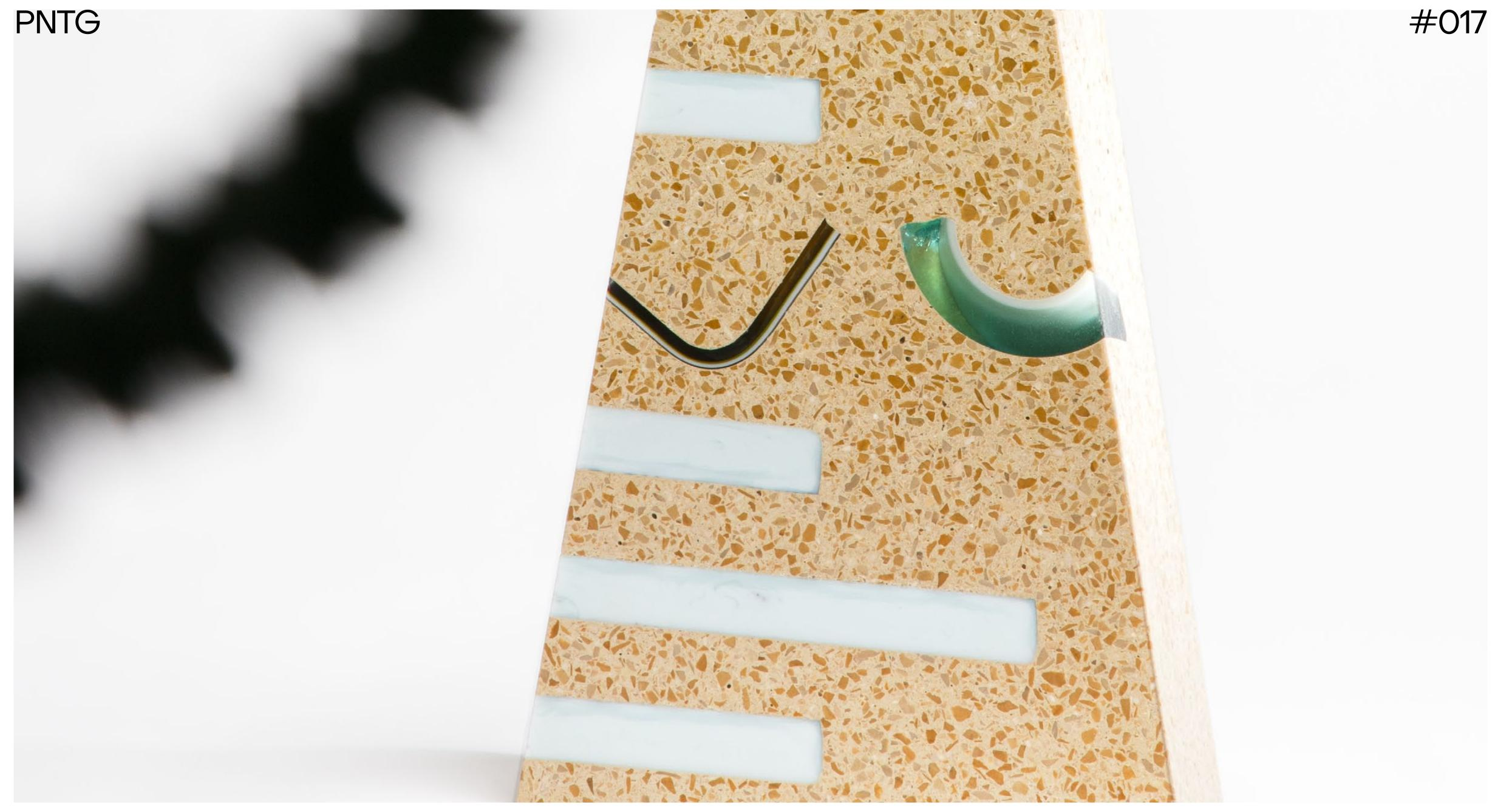
PNTG #010, 2021 DYPTICH TRANSFORMED INTO A DINING TABLE BASIS RHO - MULTICOLORED, PROCESSED GLASS WASTE IN CAST STONE
